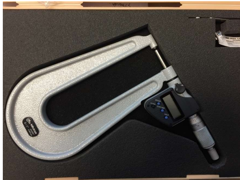
Figure 6.4 Wide mouth caliper used for measurement of the flange
